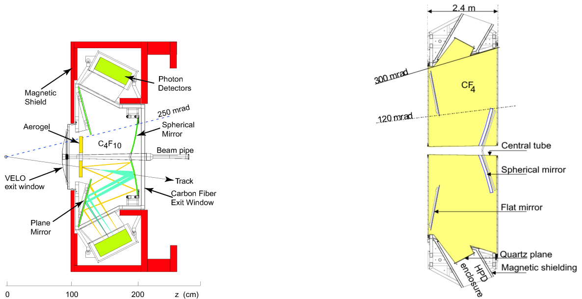
Figure 3.8: Schematic layout of the RICH1 (left) and RICH2 (right) detector [70].
