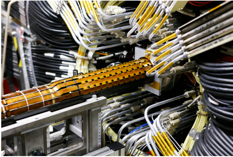
Figure 4.5: A photograph of the IBL being inserted into the center of the ATLAS detector around the LHC beam-line [52].
