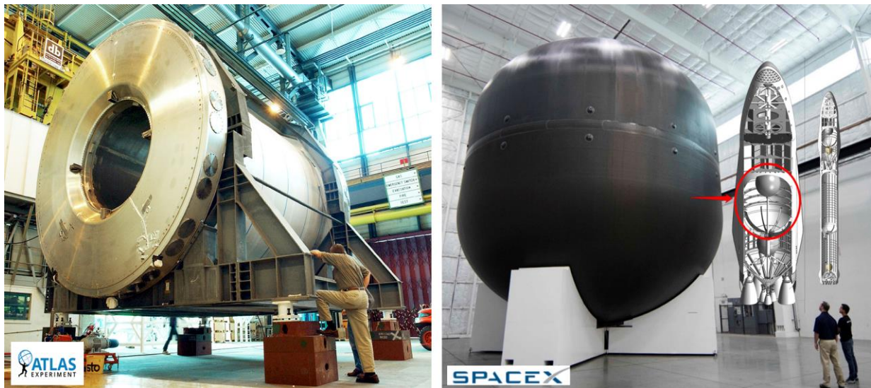
Figure 19: Left: ATLAS Liquid Argon Hadronic Calorimeter Cryostat in Aluminium Alloy. Right: SpaceX ITS LOx cryotank in Carbon Composite.
