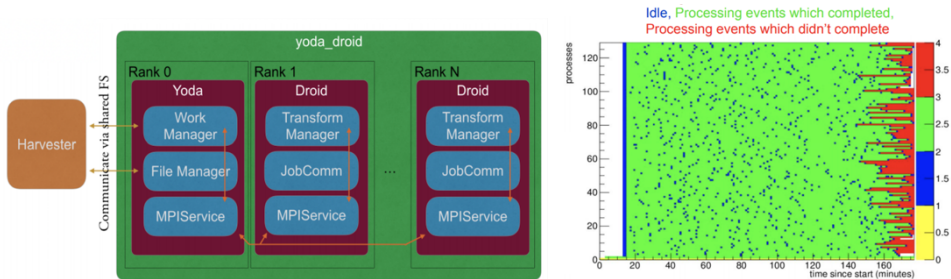
Fig. 5. a) Yoda schematic. b) Example of event level processing inside a node
