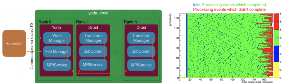
Fig. 5. a) Yoda schematic. b) Example of event level processing inside a node
