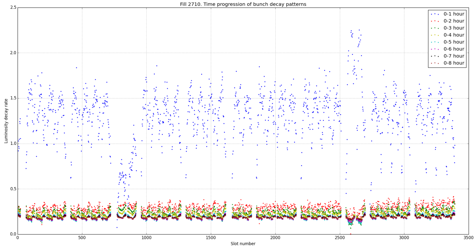
FIGURE 5.4: Luminosity decay rate ( \lambda ) dependence on the long-range beam-beam interaction during the 2012 LHC run [100]. The lifetimes of the bunches depend strongly on the bunch position (or slot number) in the train and the luminosity decay rates are the largest in the first two hours of the fill.
