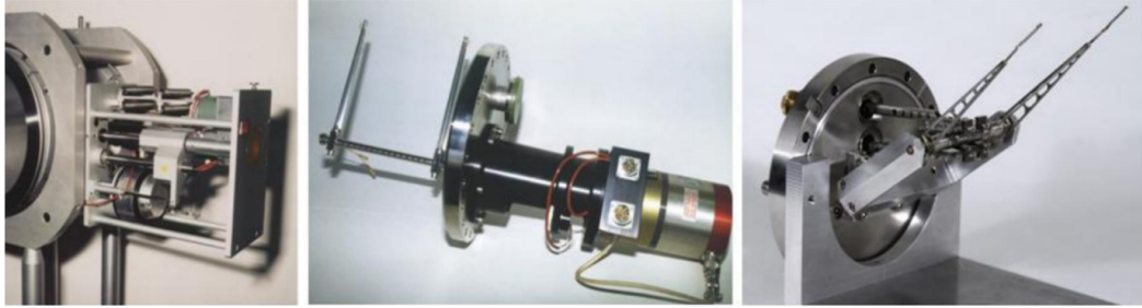
Figure 2.1 – Beam wire scanners architectures at CERN: Linear (left), Rotational (centre) and Rotational fast (right).
