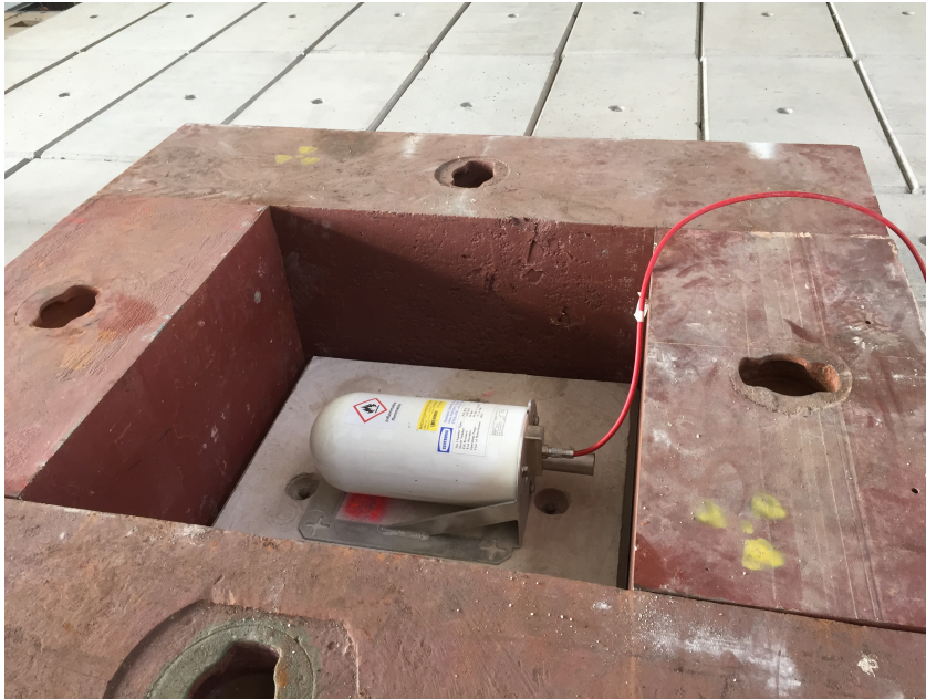
Figure 7.21: Measuring the attenuation length of barite concrete with an hydrogen-filled ionization chamber (IG5-H20) at the shielding material test location.
