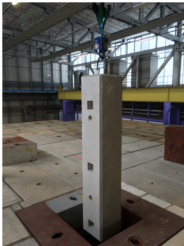
Figure 7.16: Placement of the removable sample holder concrete block, with the special designed automatic hook used only for this block.
