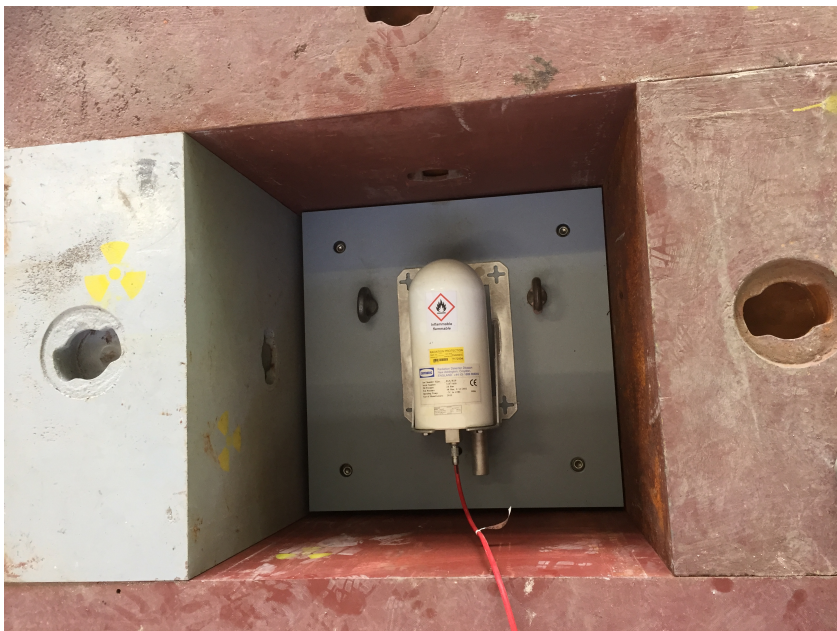
Figure 7.22: Measuring the attenuation length of cast iron with an hydrogen-filled ionization chamber (IG5-H20) at the shielding material test location.
