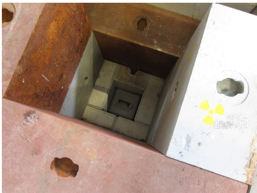
Figure 7.18: Final irradiation position of the removable sample holder concrete block.
