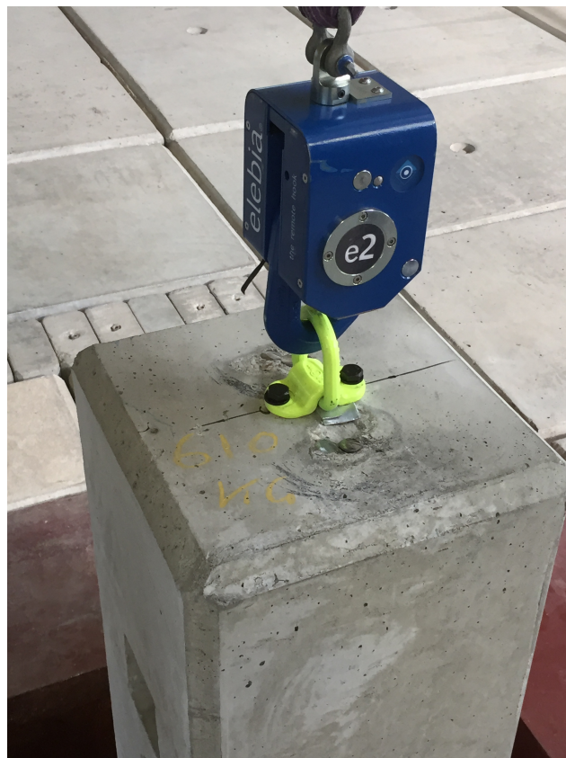
Figure 7.2: The remote controlled hook used for the manipulation of the removable sample holder concrete block.
