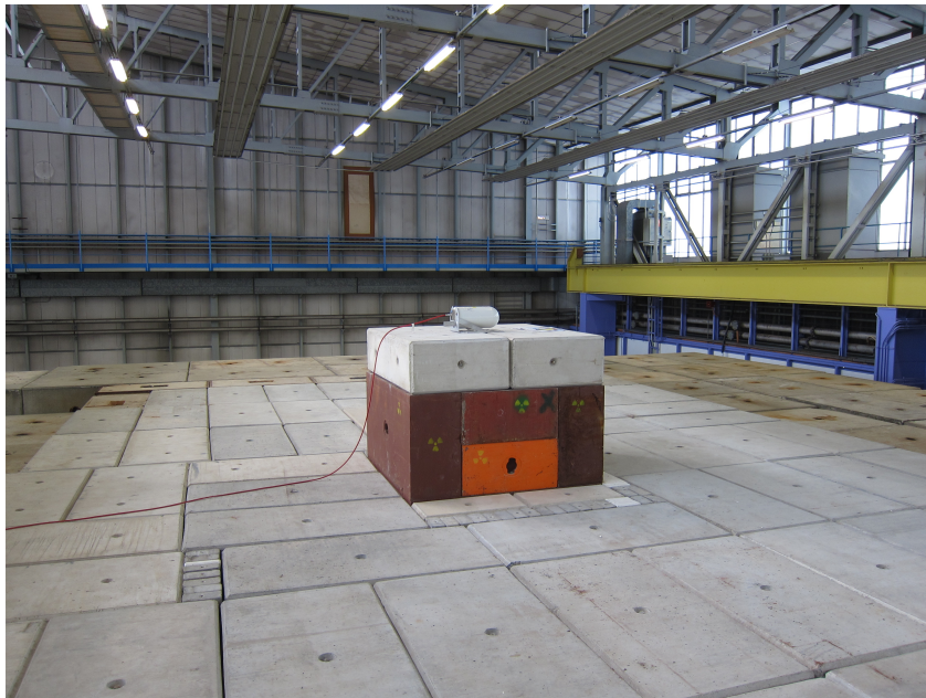
Figure 7.20: Nominal configuration of the CSBF, with 80 cm of iron and 40 cm concrete shielding. An hydrogen-filled ionization chamber (IG5-H20) is placed on top of the shielding in order to routinely monitor the radiation fields.
