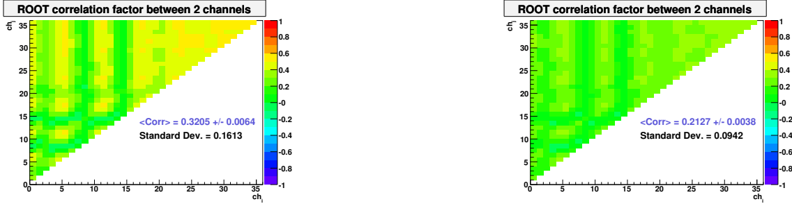
Figure 17: Layer 8, stave 2, module 3, after global corrections, and after global and SIPS corrections.
