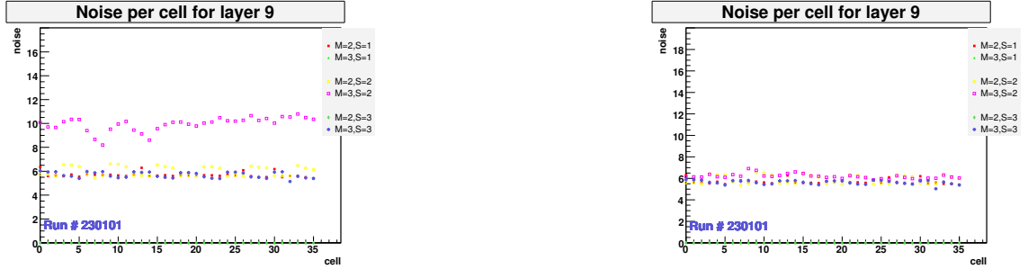
Figure 20: Layer 9, mean noise observed per wafer before any corrections, and after all corrections.
