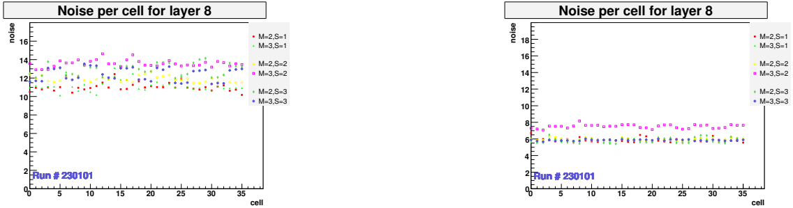
Figure 18: Layer 8, mean noise observed per wafer before any corrections, and after all corrections
