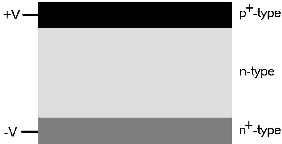
Figure 2.5: Schematic of a semiconductor detector, highlighting the electrode doping. A positive and negative bias are applied to the p-type and n-type electrodes (a forward bias).
