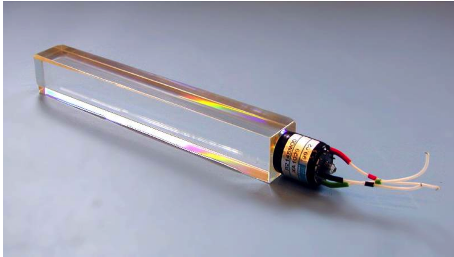
Figure 3.3: A lead tungstate ECAL crystal attached to the photodetector used to read out the light produced in the scintillating material.
