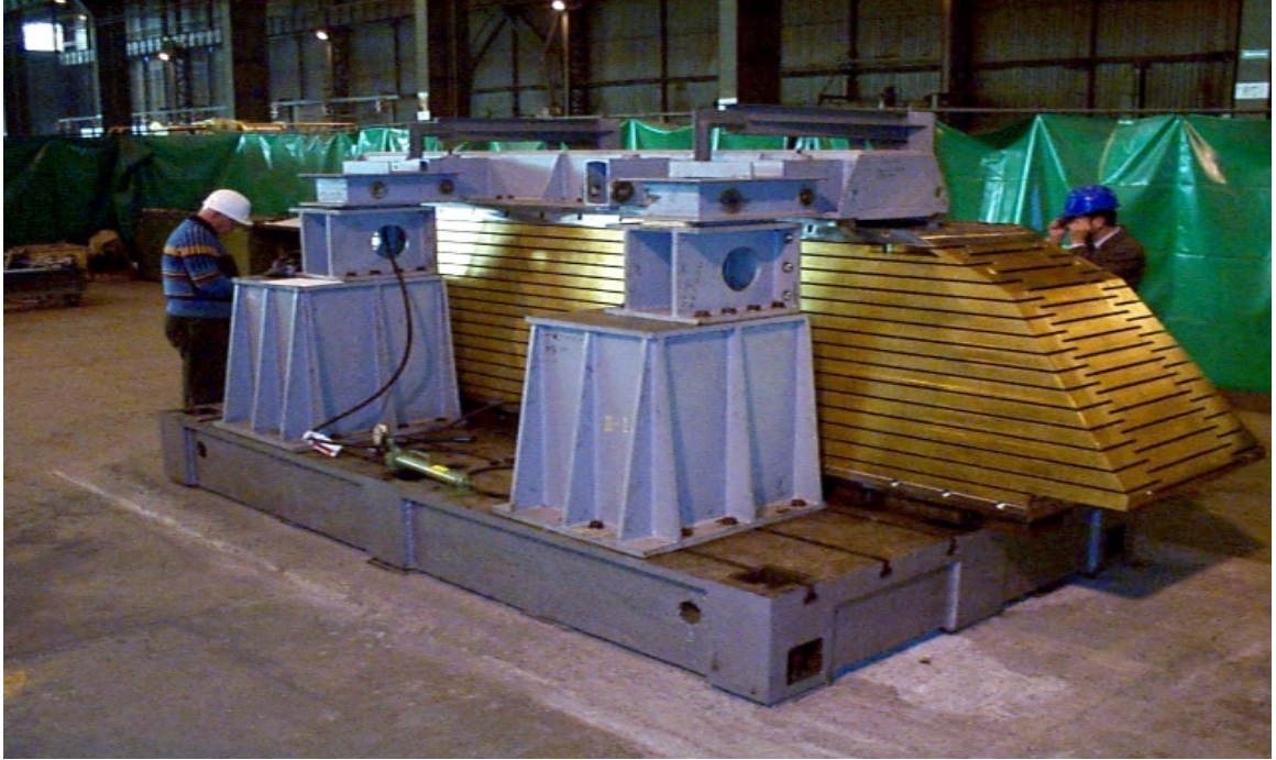
Figure 3.5: A single HCAL wedge in a test stand. The individual layers of brass absorbers are clearly visible.
