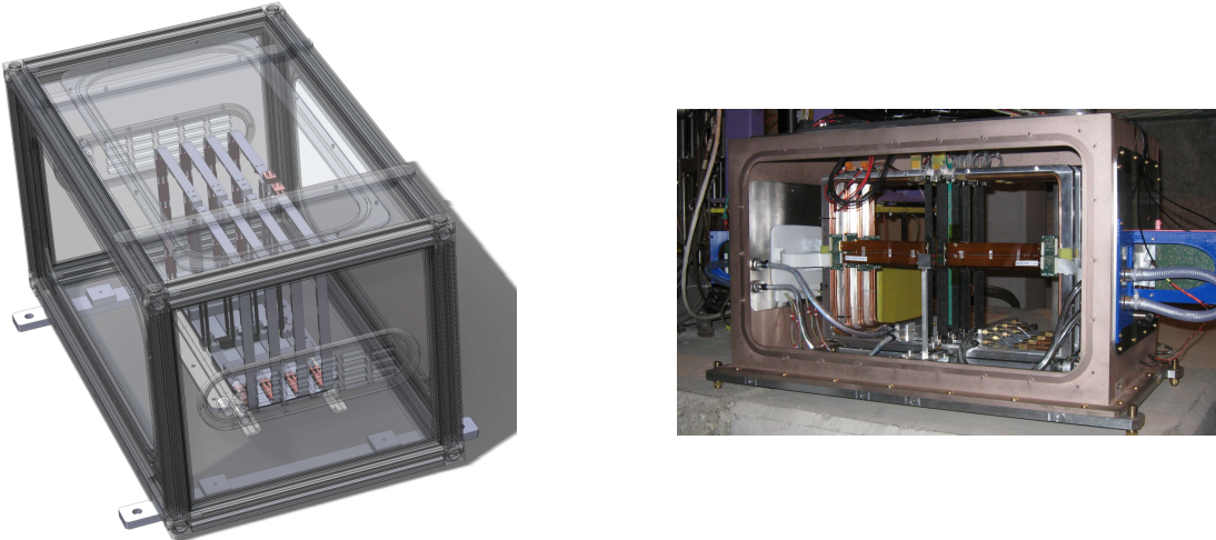
Figure 16: The final project ( Left ) and the photo ( Right ) of the Small-Acceptance Vertex Detector. Figure from Ref. [24].
