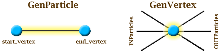
Figure A.2: Graphical representation of particles and vertices in the HepMC event record. Both object classes are interconnected through methods as indicated in the Figure, allowing for an easy navigation along particle lines via vertices.
