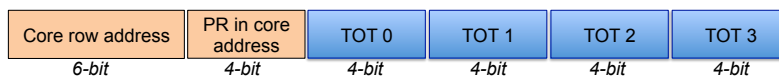
Figure 5.22: Data packet propagated at the core column level for the DBA. ToT data are propagated by DataOut signals, whereas the address of the pixel region in the core and the core row are fed to the RowOut signals.
