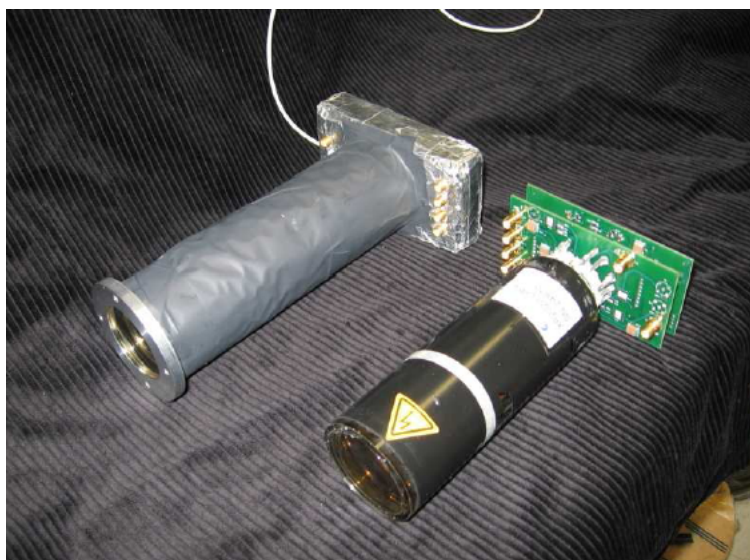
Figure 4.4. A TCD PMT before and after being potted and wrapped (with mounting ring also attached).
