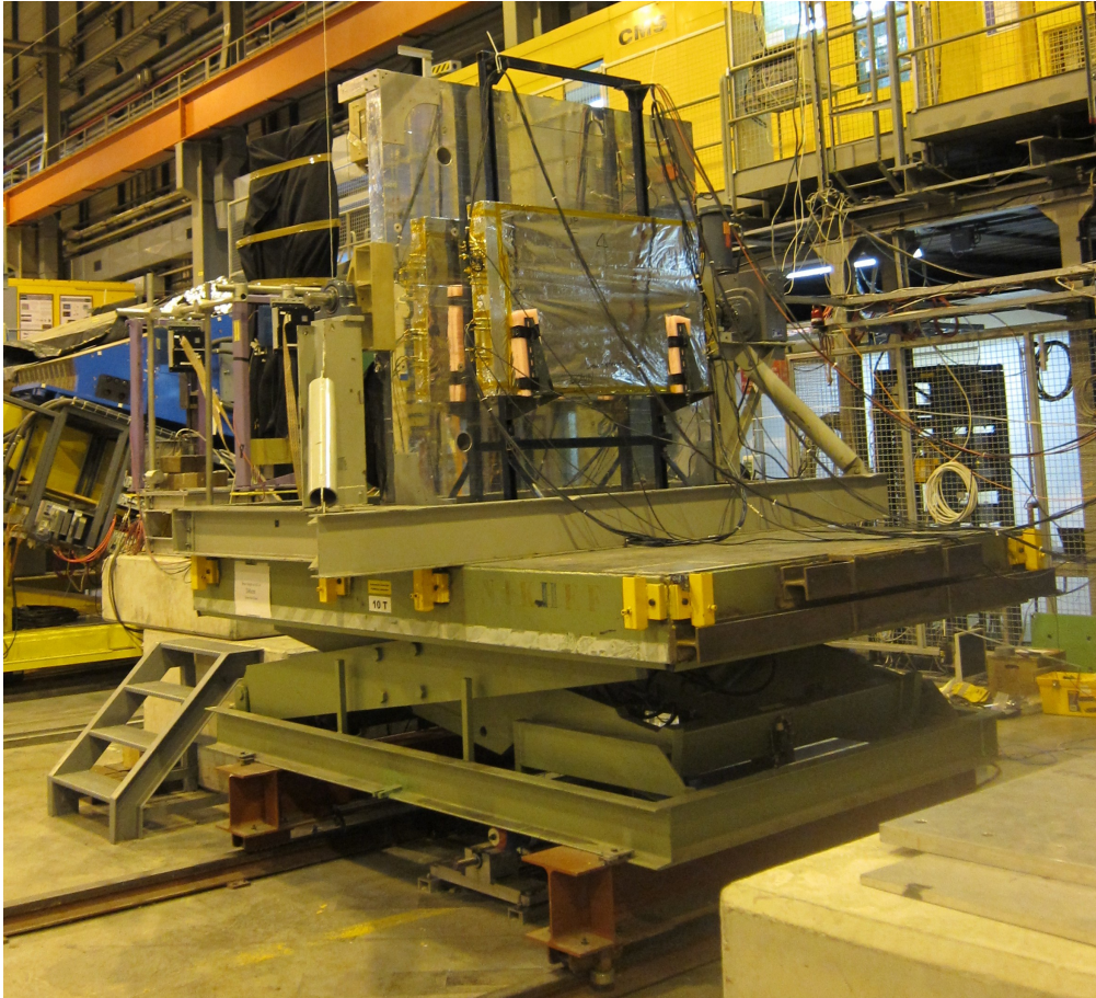
Figure 6.7. The prototype BSD detector mounted behind the ISS-CREAM instrument calorimeter pallet in the CERN H2 beamline.
