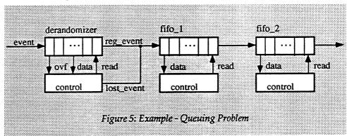
can accept a limited amount of event data. Whenever the buffer contains data, they will be read. This takes a certain (for this example fixed) amount of time per registered event (readout delay). Events which occur while the buffer is full will be lost.
