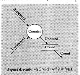
previously mentioned dataflow description elements. This allows one to describe the timing and control behavior of a system. In Figure 4, "Increment" and "Decrement" belong to the timing-and-control category, while the other elements are data-flow elements. A further evolution was to combine characteristics of these notations and methods into a
