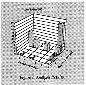
events, and (ii) pushing the readout delay to values below 9 µs will only result in somewhat marginal improvements. In addition to these results, the simulation helped to detect a potential problem with regard to emptying the buffer. Under certain circumstances a race condition was observed. Event data could enter the buffer unregistered and "clog" it.
