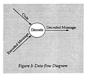
of a class of methods and notations to do so is *Structured Analysis* <sup>[3]</sup> (DeMarco). Its main elements are processes, data-flows, datastores, sinks, and sources. With these elements one can describe a system in a form which is known as data-flow diagram (Fig. 3). But, dataflow diagrams based on structured analysis do not
