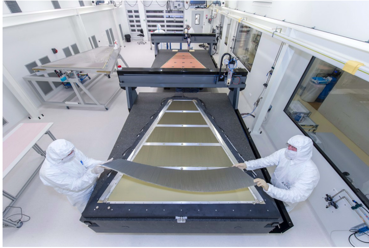
Figure 2: The ATLAS team in the Saclay clean room building a large area resistive micromegas module for the ATLAS New Small Wheel Upgrade [19].
