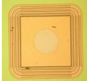
Fig.3.17 Picture of a diode with total area of 6x6 mm 2 and 4 contactable GR's structure (LAL design)
