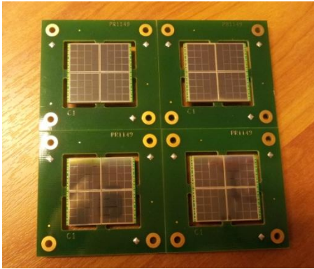
Fig. 5.56 Picture of 4(2x2) elementary modules, each of 4(2x2) arrays mounted on PCB's, building the full SIPMED camera
