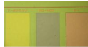
Fig.3.6 Picture of test-structure dedicated to doping profiles measurements; the three zones have different types of implants: moderated p-spray implant (left zone), standard p-spray implant (middle zone), n^+ implant (right zone); a boron implant exists on the whole backside of the sample
