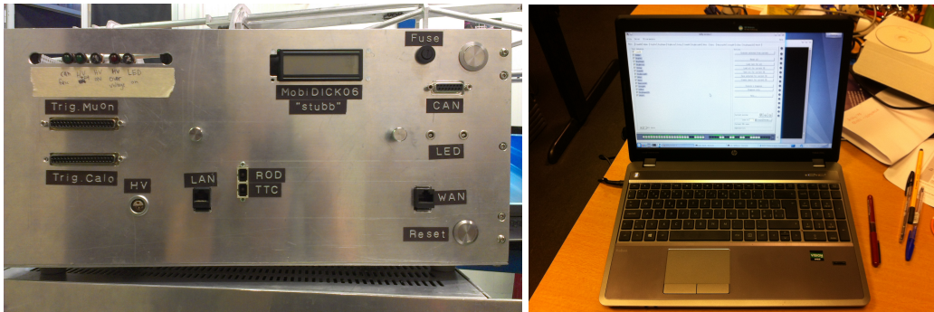
Figure 3.18: The MobiDICK4 hardware box (left) and the associated lepton (right). They communicate through an Internet which access to the GUI interface implemented in the MobiDICK4 [18].
