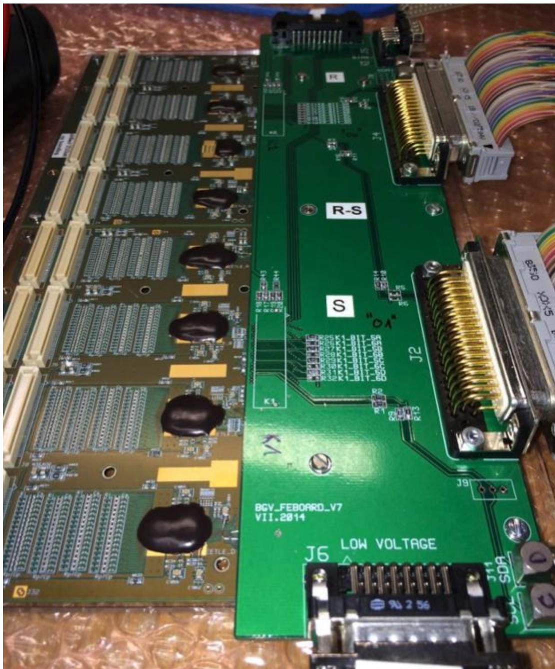
Figure 3.12.: Photo of the FE board of one side of the SciFi detector module. On the left are the connectors for the flex cables from the SiPMs, right of the connectors are the attenuation circuits. The black spots cover the Beetle chips. The green board (marked “R-S”) in the centre receives the voltage to power the Beetles and SiPMs. In addition, it receives and transmits control signals and trigger/clock signals from and to the Beetles. The flat cables on the right side are 7 m long data cables which send data from the Beetles to the RPT boards.
