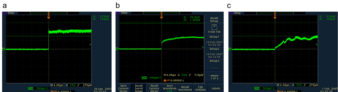
Figure 3.8: STO behaviors of an VCSEL: no STO (a), mild STO (b), and severe STO (c).
