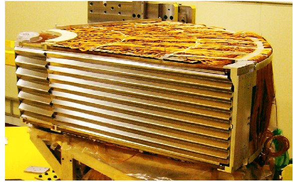
Figure 3.10: Photo of EMEC wheel under construction. Both inner and outer wheels are visible [51].
