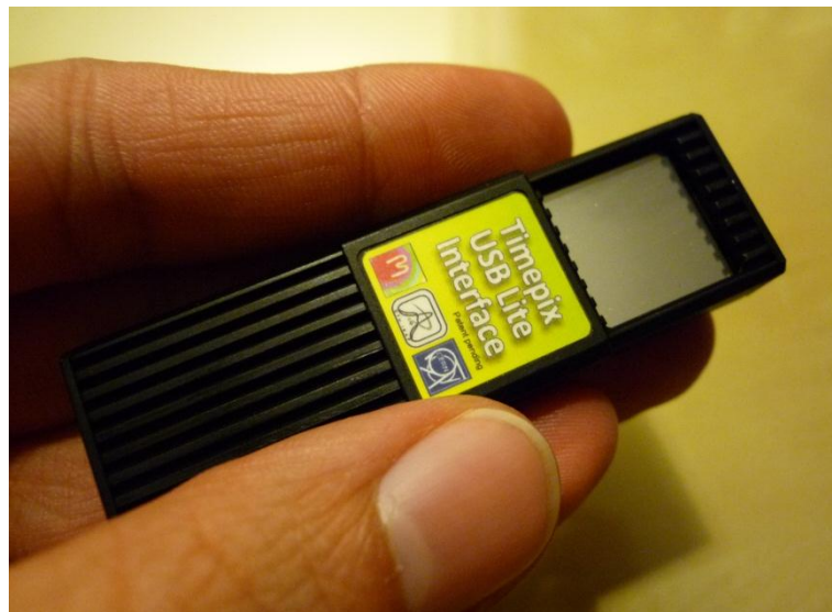
Figure 18. USB Lite interface is the step in further readout interface miniaturization where dimensions of the whole setup has been reduced to 15 mm × 60 mm (25% out of it is the active area of the Medipix2 detector).
