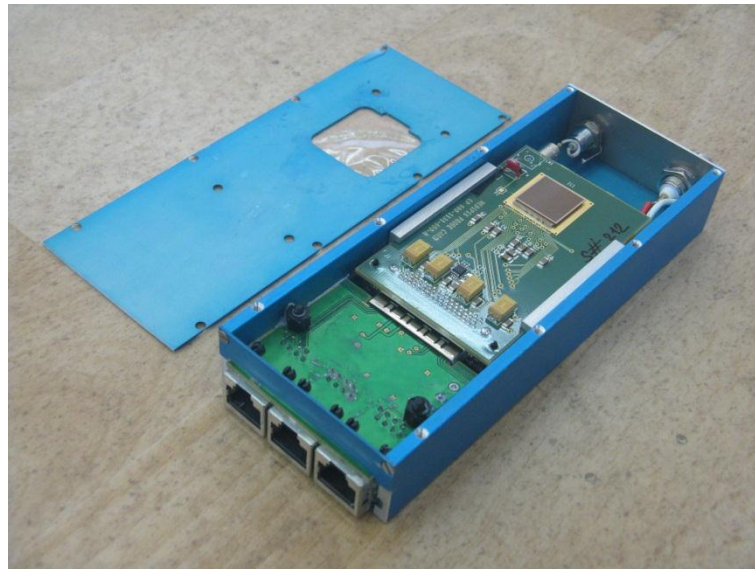
Figure 30. ATLAS-MPX detector (Medipix2 detector without the neutron conversion layers) mounted in the duralumin box.
