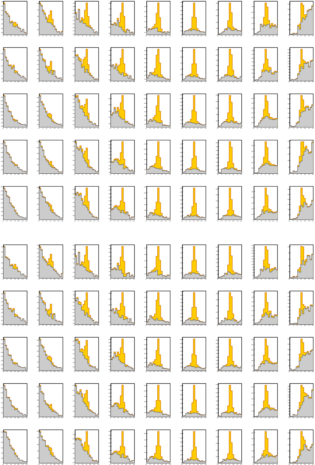
Figure 6.7: Invariant mass spectra ( 60 \text{ GeV} < M_{\text{tag,probe}} < 120 \text{ GeV} ) in bins of E_T (horizontal) and |\eta| (vertical) to determine the reconstruction efficiency via the tag-and-probe method. By fitting, the contribution of signal (orange) and background (grey) in each bin is determined (cf. Equation 6.14). Top: double-differential denominator. Bottom: double-differential numerator.
