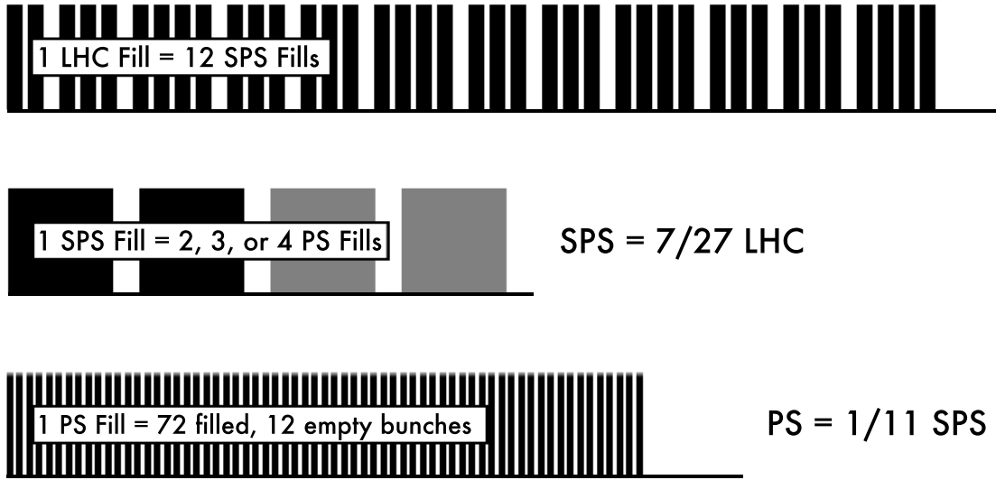
Figure 2.3: Schematic drawing of the 25 ns filling scheme used for nominal pp collisions in the LHC. Inspired by [68].
