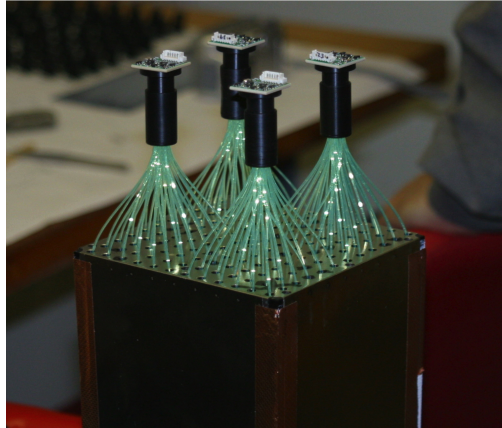
Figure 1.5: The basic module of EMCAL at ALICE. Taken from [16] p.11.
