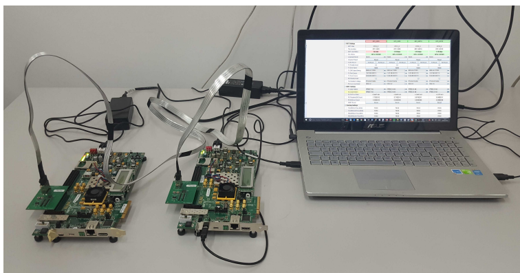
Figure 5.37: Set up for testing the transmission quality of the miniSAS cable.
