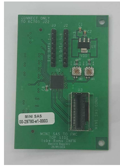
Figure 5.38: The FMC mezzanine board.
