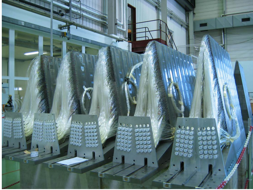
Figure 3.11: Hadronic Forward (HF) calorimeter wedges with quartz fibers stretching from absorber steel blocks (CERN, 2016).
