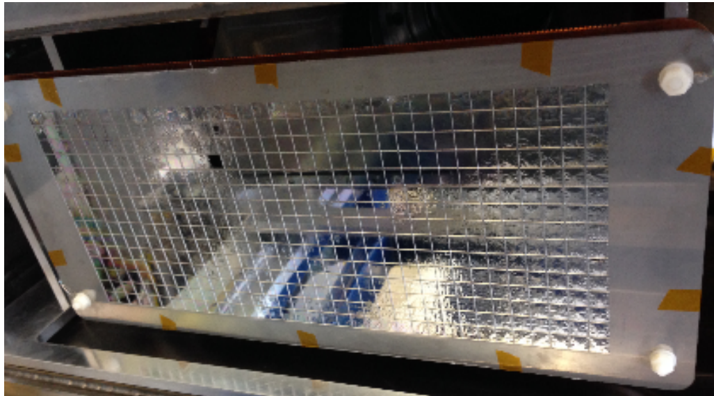
(a) A photograph of the electron emitting foil of the STOP detector.
