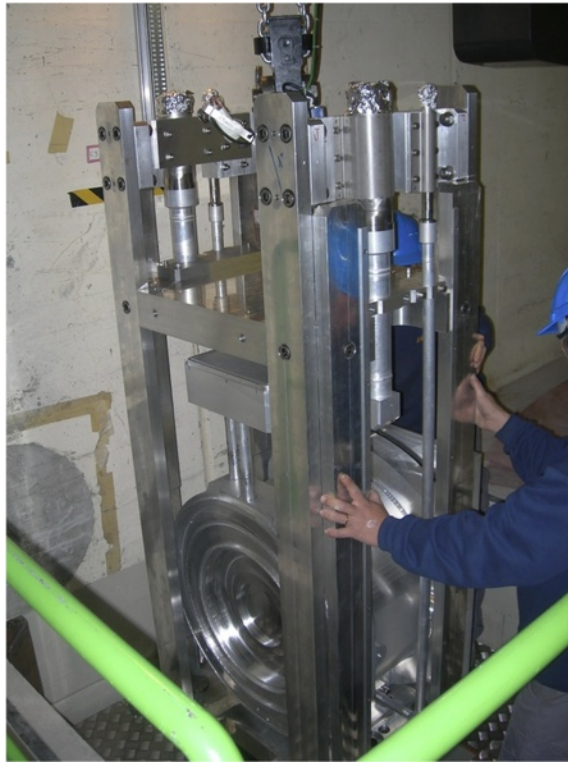
Figure 3.2: The current lead spallation target used at n_TOF, pictured during its installation.
