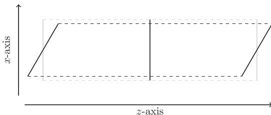
Figure 5.7: The coordinate system is defined by the outermost planes in the tracker system. If the planes are assumed to be parallel to the global x -axis as indicated by the gray vertical lines, but are in fact rotated around the y -axis, as illustrated by the black lines, the global x -axes will be compressed. The length and pitch of the plane in the middle of the system will appear larger than what they actually are if measured in the compressed coordinate system. In this case the numerical alignment will suggest a scale factor larger than one for the middle plane.
