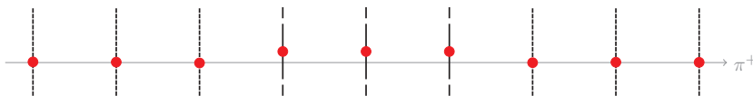
Figure 5.13: Illustration of error correlation in a detector system with three planes with little charge sharing surrounded by planes with better resolution. The vertical black lines represent readout channels, the red dots are the measurements and the horizontal line is the particle trajectory. The errors in the center planes are systematic and correlated in events with no charge sharing.
