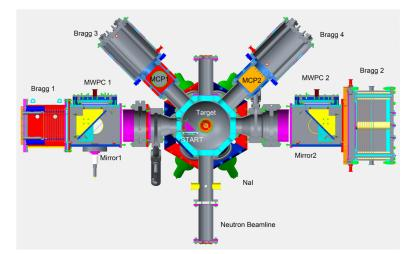
Figure 1: STEFF in the new configuration for EAR2 shown as a section in a vertical plane through the centre-line of the spectrometer. The neutron beam travels from bottom to top in the figure. The TOF arms contain the START detector and two STOP detectors. The short arms have STOP detectors (MCP1 and MCP2) but no STARTs.
