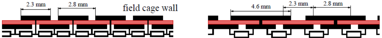
Figure 6: Possible configurations for the case of double sided copper strips.
