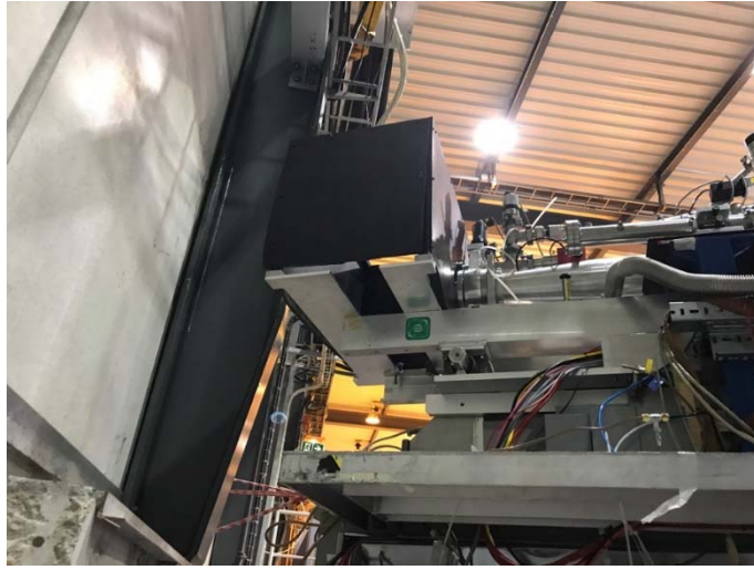
Figure 22: Bottom-up view of the KWISP 2.0 sensor installed on the CAST beam-line with full shielding. The hypothetical chameleon beam impinges from the right. The X-ray telescope external tube is visible at center-right.
