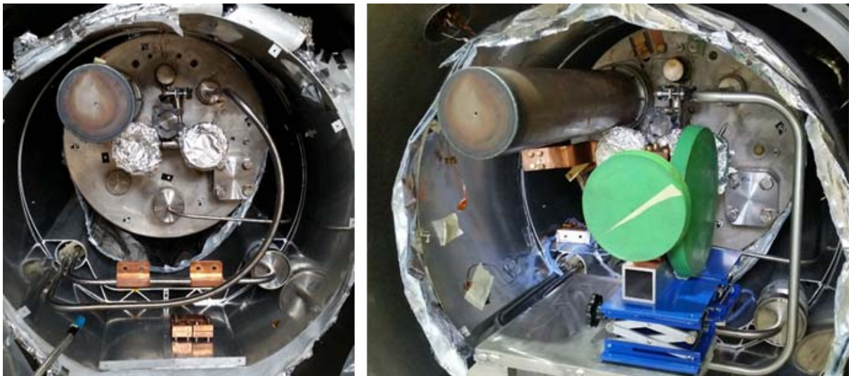
Figure 6: The modification of the return pipe of the CAST magnet was necessary to fit two signal feedthrough vessels for the two types of cavities.
