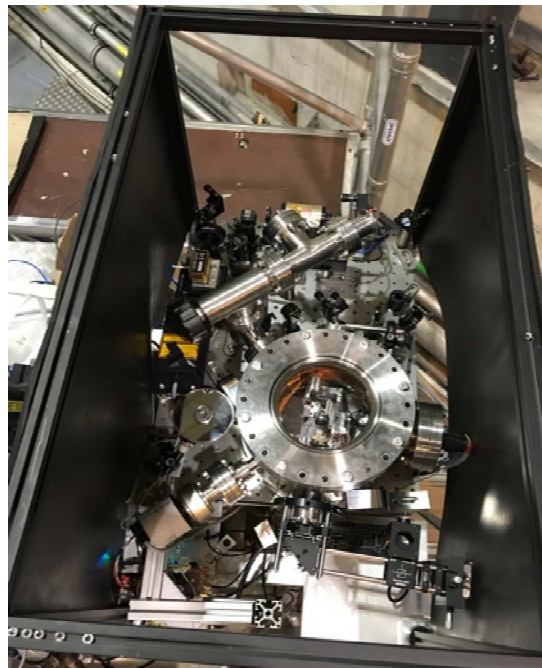
Figure 21: Top view of the KWISP 2.0 sensor installed on the CAST beamline with the shielding removed. The vacuum chamber holding the sensing membrane is visible at the center, with the chopper wheel at its left. The hypothetical chameleon beam impinges from the left after passing through the X-ray telescope
