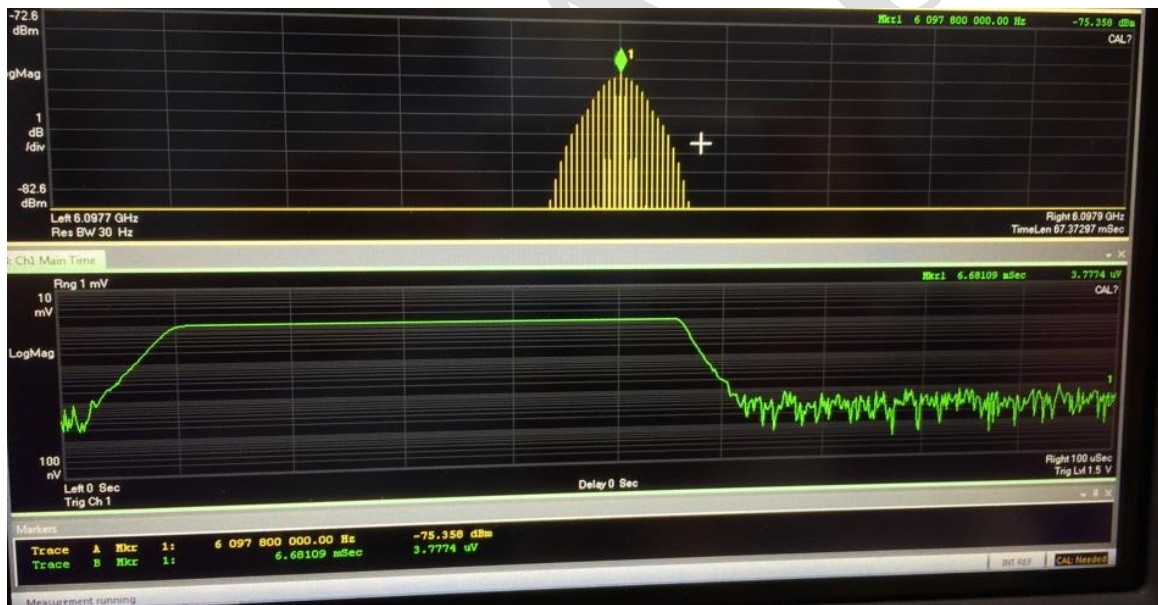
Fig 6 – The signal Analyzer representation in FFT mode of a “20 KHz axion signal width”. Frequency domain on the top panel, time domain on the bottom panel.
