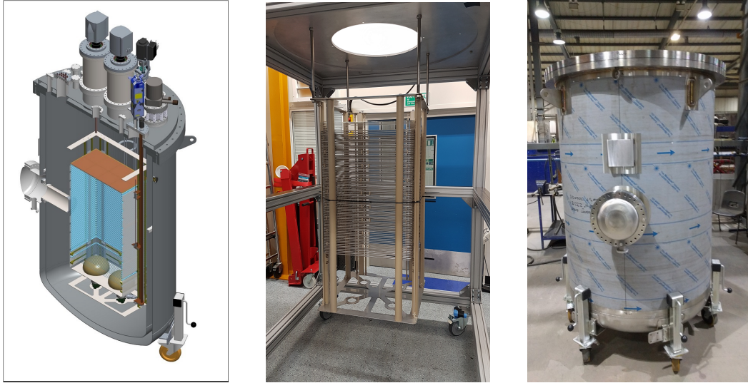
Figure 1: (Left) Section-view schematic of ARIADNE, showing the TPC field rings (blue), 2 of the 4 PMTs (bottom, gold), THGEM (brown) and beam plug (far-left, silver) all located inside the vacuum-jacketed cryostat, with the cryocooler head (top-right, dark grey) and 2 of the 4 EMCCD cameras also visible on top of the detector. (Centre) View of the TPC suspended from a temporary construction frame. (Right) The ARIADNE cryostat and beam plug, prior to being shipped from the manufacturer to the University of Liverpool.
