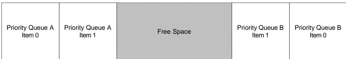
Figure 28: Allocation of memory between the two priority queues with free space between
