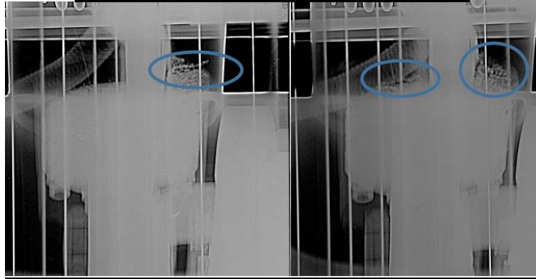
Fig. A-1: X-ray image of the ‘half-moon’ connector of the affected magnet during EYETS 2016/2017: before and after burning of the fault.
