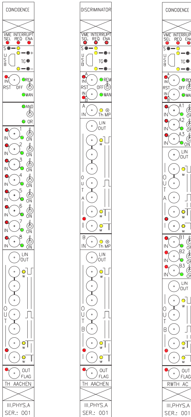
Figure C.3.: The front plates of the designed VME-modules for the final VDC system at CERN [Hil07].
