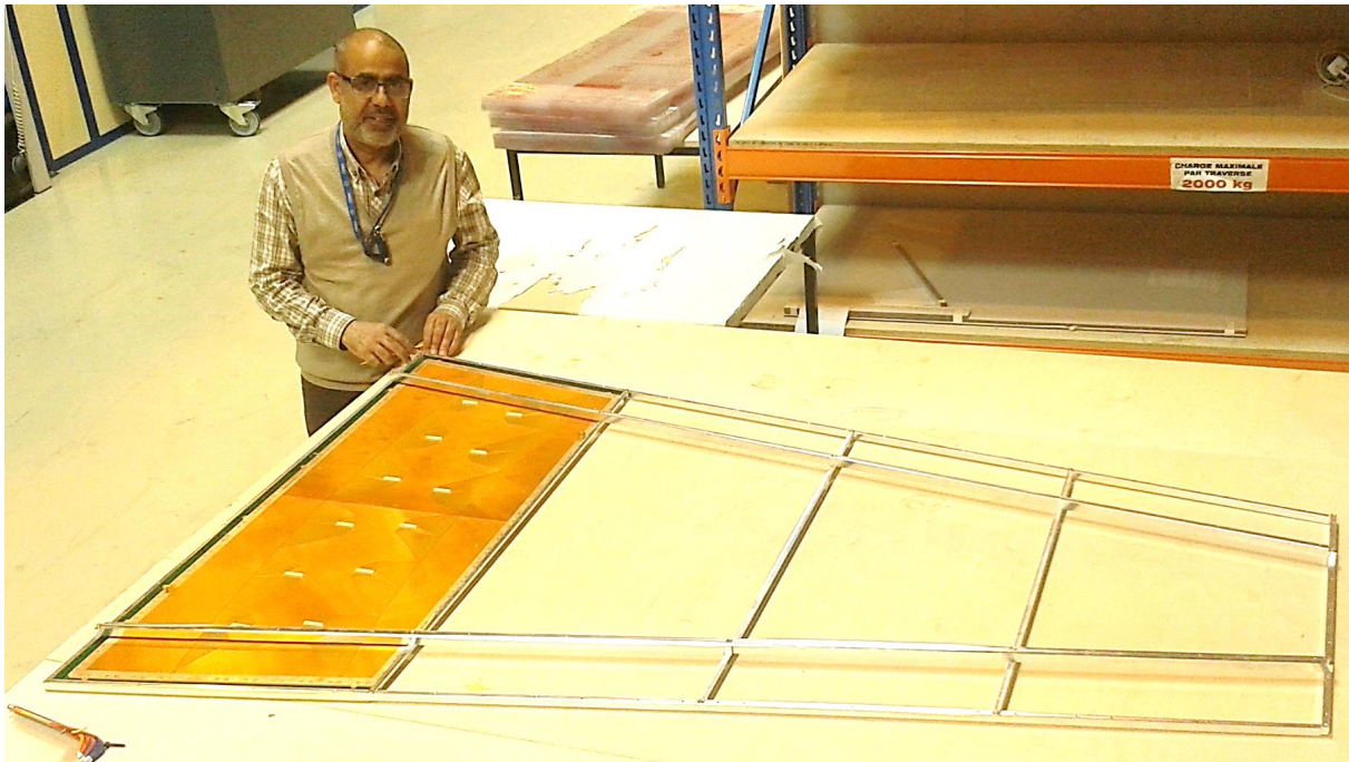
Figure 6.38: Prototype of GE2/1 aluminum coupling frame; the M4 prototype module is fixed on the structure in its final position.
