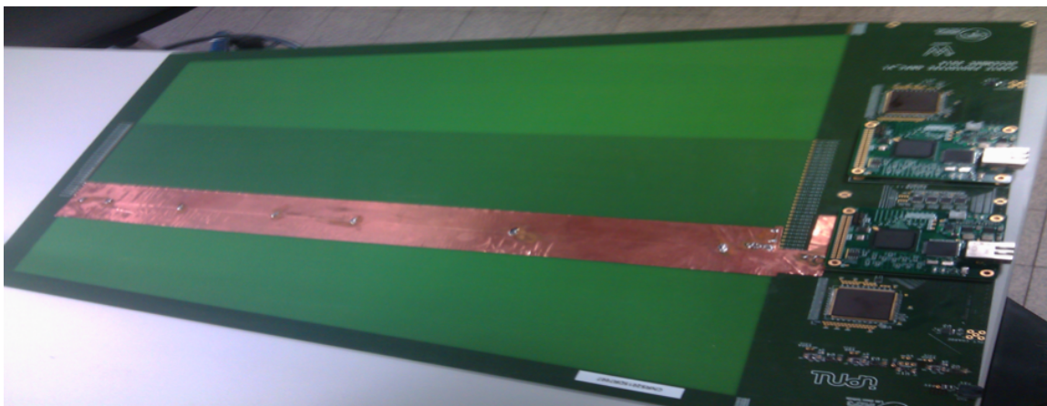
Figure 5.25: Picture of the preliminary version of the ASU with the final version of the FE board embedded on it, used to test the new readout schema. Pickup strips are placed in the middle.
