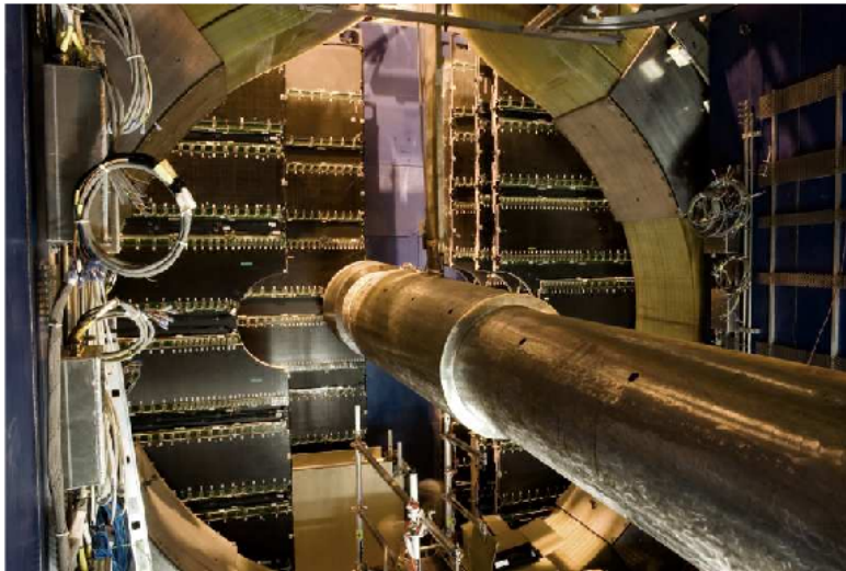
Figure 3.11: Layout of the station 2 of tracking system. Readout electronics is distributed on the surface of a quadrant structure.
