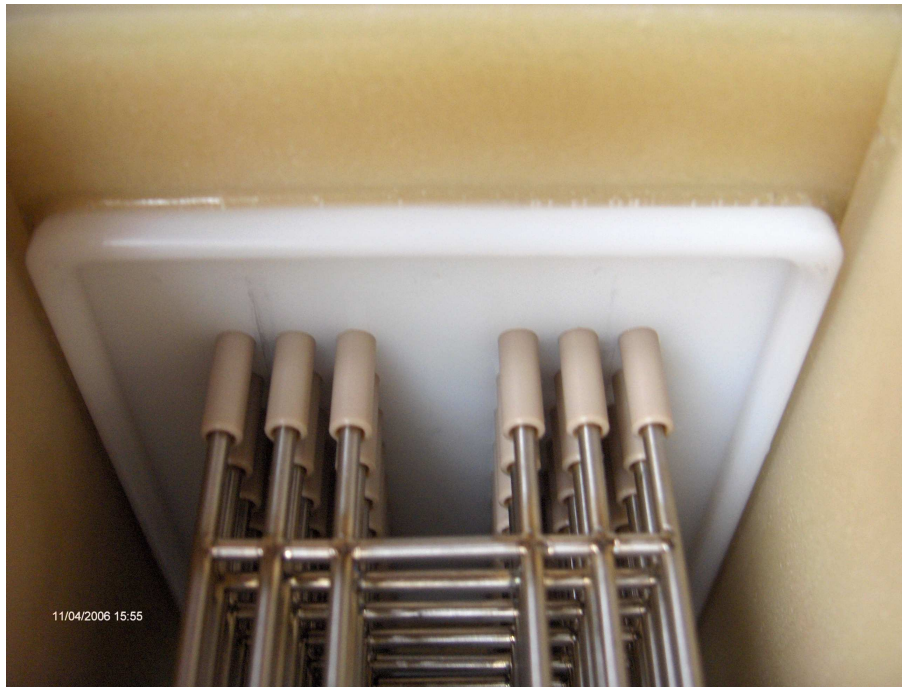
Figure 7.4: The field shaping electrodes fixated in a Polyamid-plate that is inserted in the chamber walls. The electrodes are additionally protected by small insulators made of PEEK.
