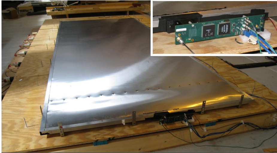
Figure 6.13: Photo of CRT module. The inset shows the front-end board attached to the PMT and module. The two large chips are the MAROC2 and an Altera FPGA.
