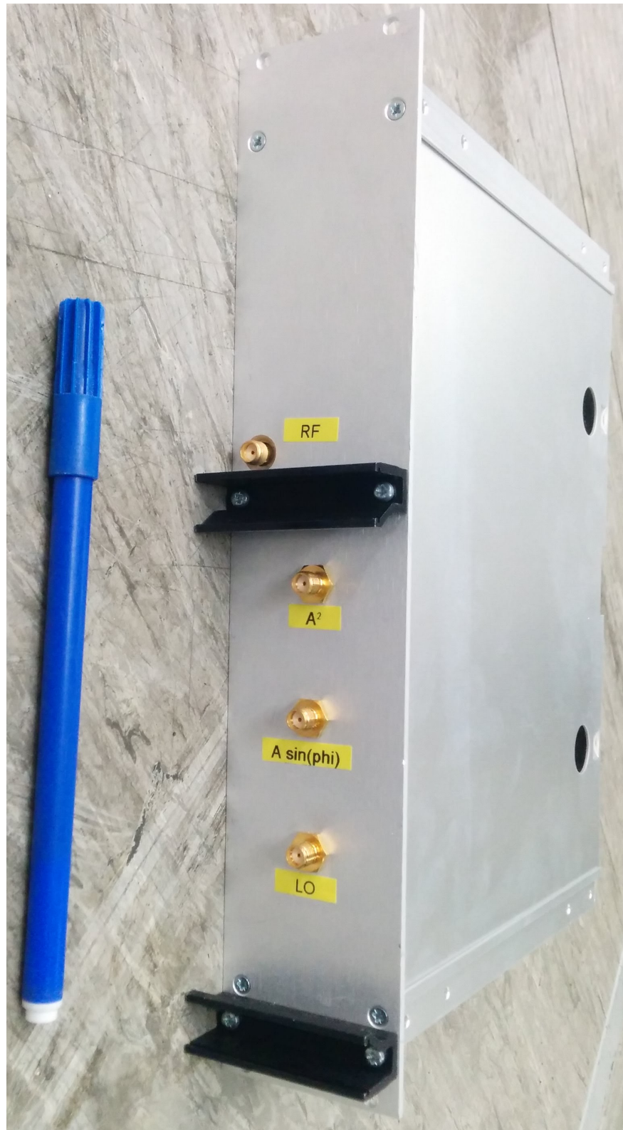
Figure 3.5: Front panel of the phase monitor electronics boxes containing the mixers and diodes. The connectors labelled LO and RF take the signals from the LO source and the phase monitors respectively. The connectors labelled A^2 and A \sin(\phi) are the diode and mixer outputs respectively.
