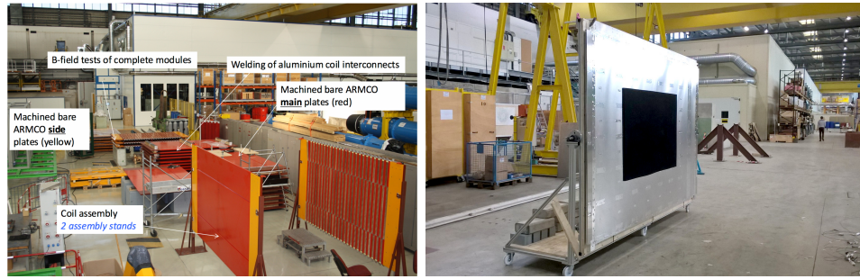
Figure 3: (Left) The Magnet assembly zone, (Right) A scintillator module.
