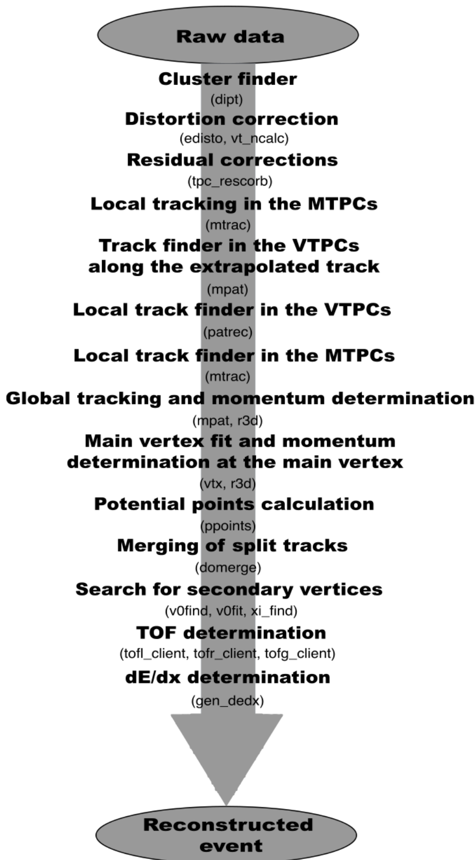
Figure 3.12: The NA49 reconstruction chain. Figure taken from [28].
