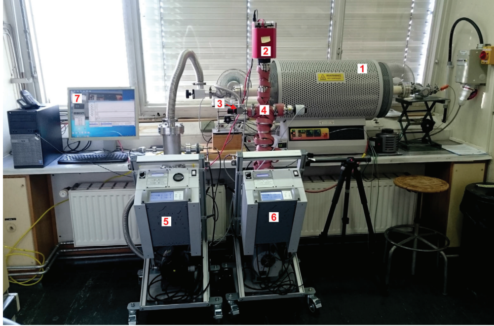
Figure 2.4 – Setup used for the residual gas analysis which consisted of oven A (1), the RGA unit (2), the valve connecting the oven and the RGA unit vacuum systems (3) the heating elements to bake out the vacuum system of the RGA unit (4), the oven and RGA unit pumping groups (5 and 6 respectively), the computer with the software to analyze the signal coming from the RGA unit (7).
