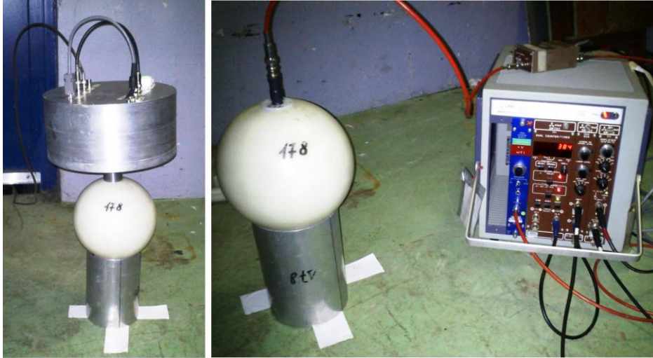
FIG. 49. Experimental set-up for the measurements performed with the 178 mm sphere at the CERN PS: BSS-LUPIN (left) and conventional CERN BSS (right).
