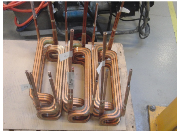
Figure 3.67. MKC coils after impregnation
