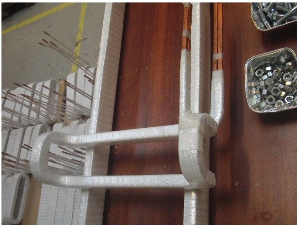
Figure 3.66. MKC coil before impregnation
